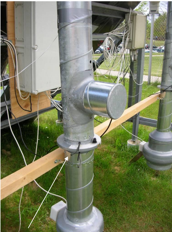
Fig.5 Iris damper with pressure ports used in the flow sensor calibration. The flow sensor is covered by the T-joint.
