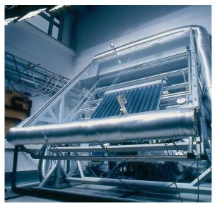
Figure 1: Solar Irradiance Simulator at Fraunhofer ISE
