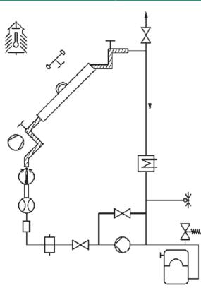
Figure 1: Example of a closed test loop. Description of the components can be referred to from the Standard.
