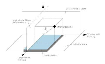
Figure 1: Longitudinal and transversal plane as reference for IAM description; Fraunhofer ISE
