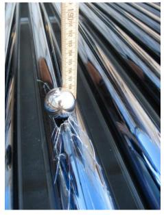
Figure 3: Damaged collector after steel ball impact test
