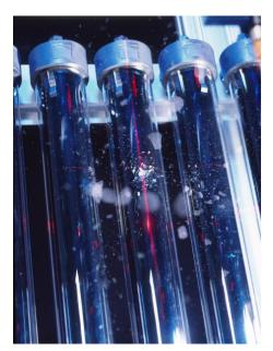
Figure 2: Collector after ice ball impact test
