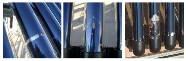
Figure 2: Damaged collectors after testing; Fraunhofer ISE
