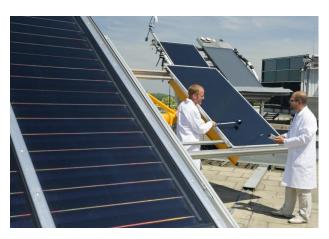
Figure 1: Test setup at TestLab Solar Thermal Systems, Fraunhofer ISE.
