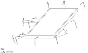
30° angle of spray nozzle with respect to the collector surface
