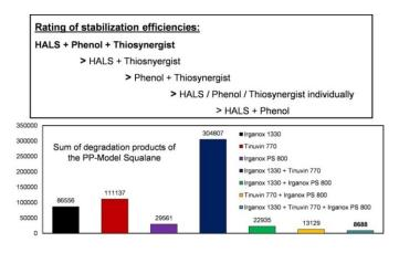
Stabilization mechanisms of the most important additive groups for long-term heat protection of polymers were investigated. A highly sensitive HPLC-MS method was developed to detect and identify stabilizers and their degradation pathways. To elucidate the longterm heat protection efficiency of different stabilizer formulations and the possible chemical reactions between different stabilization classes, several antioxidant systems consisting of HALS in combination with
