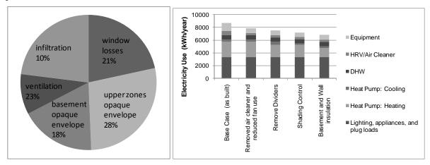
Figure 6: a) distribution of total heat loss during the heating season; b) electricity use for successive upgrades
