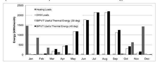
Figure 7: Comparison of thermal loads and BIPV/T useful energy output
