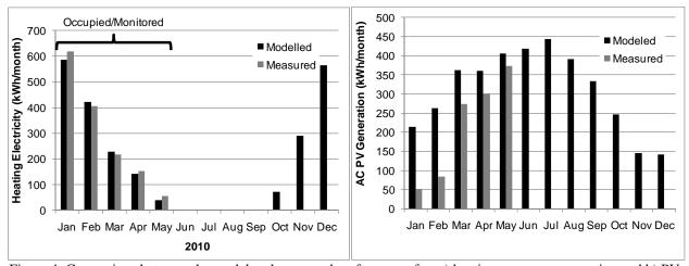
Figure 4: Comparison between the model and measured performance for: a) heating energy consumption and b) PV electricity generation
