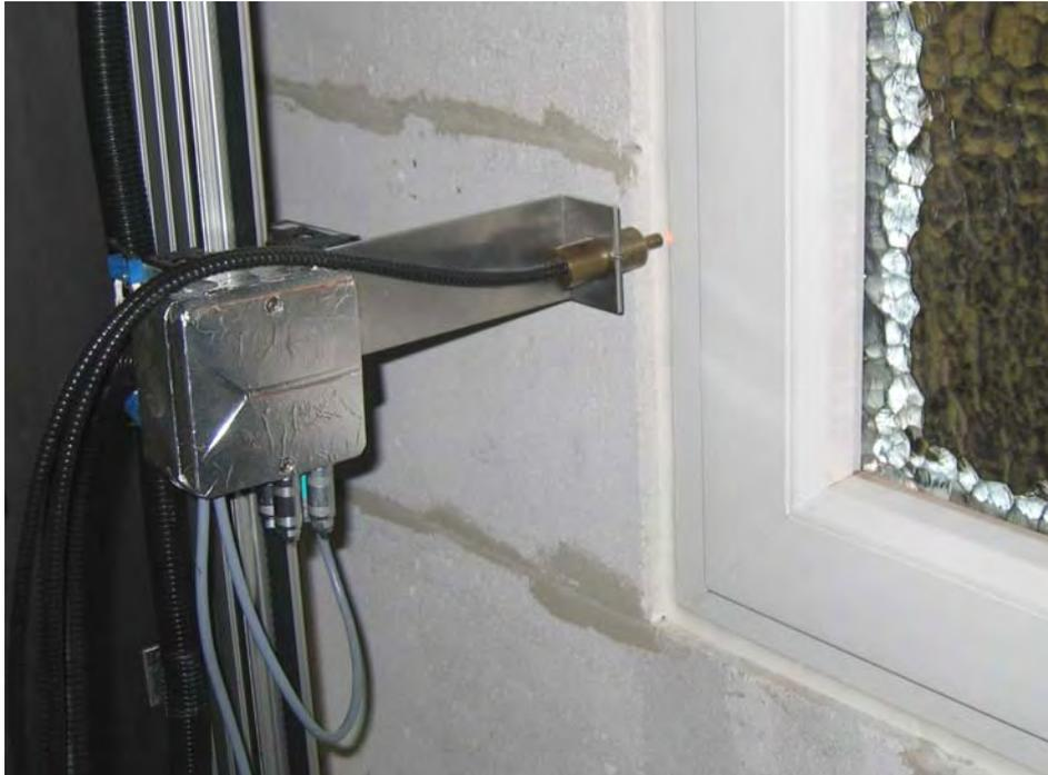
Figure 5.2: The humidity sensor mounted on the scanner
