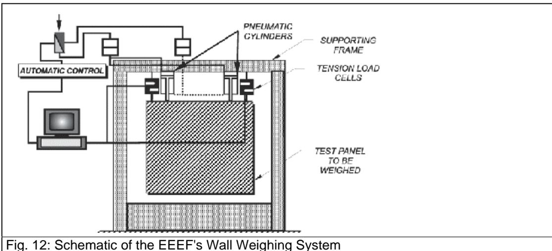
Fig. 12: Schematic of the EEEF's Wall Weighing System
