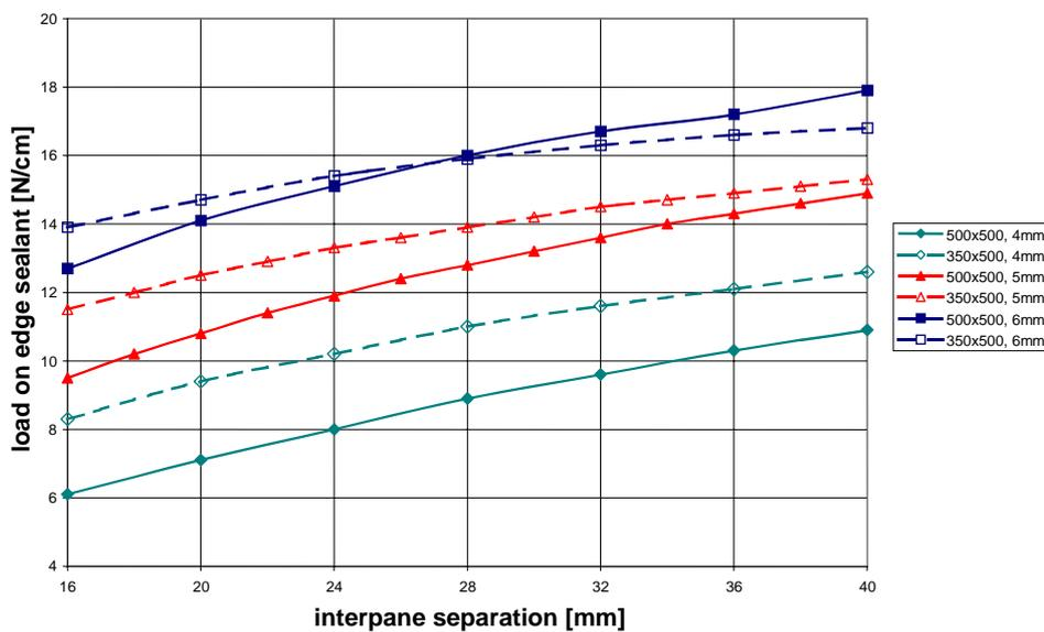
Fig. 33: Load on edge sealant against interpane separation for DGU with 4 mm, 5 mm and 6 mm glass panes, with a specimen size 350 x 500 mm<sup>2</sup> and 500 x 500 mm<sup>2</sup>
