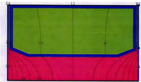
**Fig. 3: Isotherms for a Stainless Steel spacer with a conductivity of  $14.3 \text{ w/m K}$ . Thickness of metal  $0.18 \text{ mm}$ . Equivalent conductivity is  $7.15 \text{ W/m K}$**
