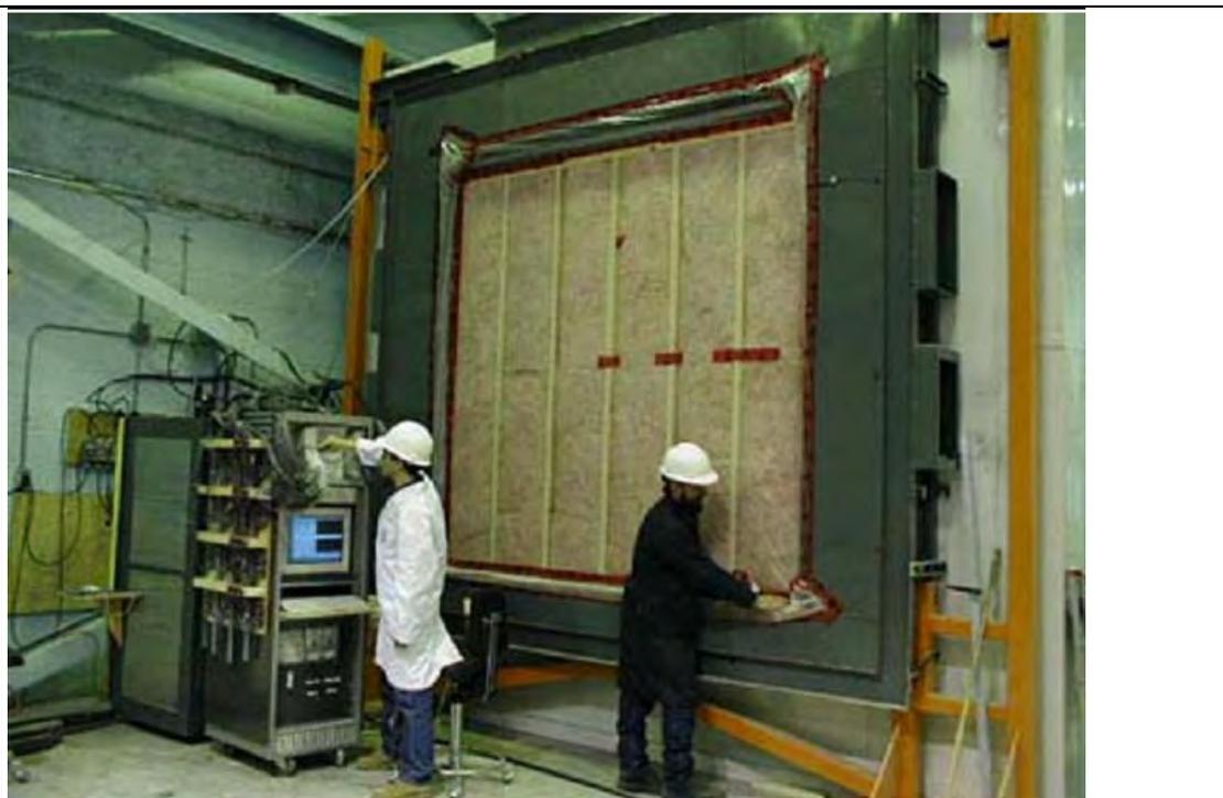
Fig. 11: Preparing a Full-Scale Wall Specimen For a Drying Experiment in the Envelope Environmental Exposure Facility (EEEF)
