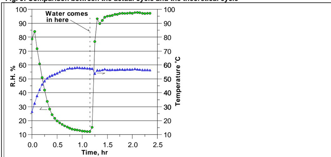
Fig. 10: Air temperatures and humidity ration during a typical cycle
