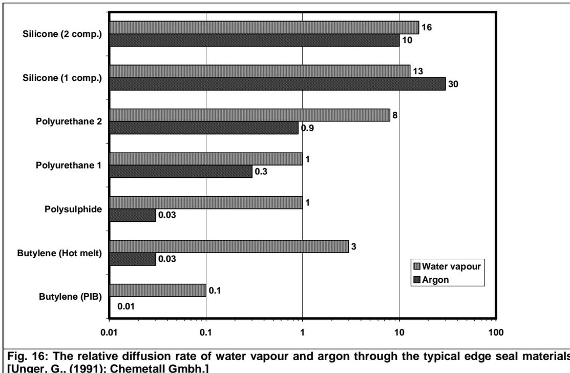
Fig. 16: The relative diffusion rate of water vapour and argon through the typical edge seal materials [Unger, G., (1991); Chemetall GmbH.]
