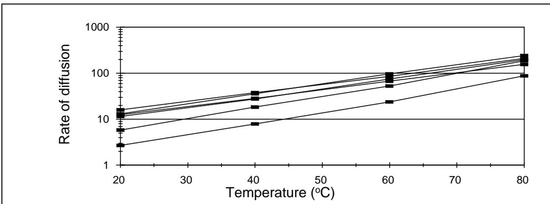
Fig. 14: The influence of the temperature on the vapour diffusion for different materials.
