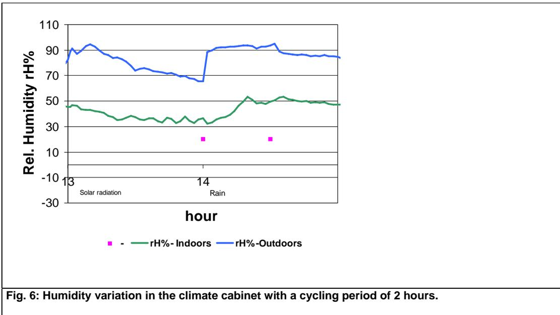
Fig. 6: Humidity variation in the climate cabinet with a cycling period of 2 hours.
