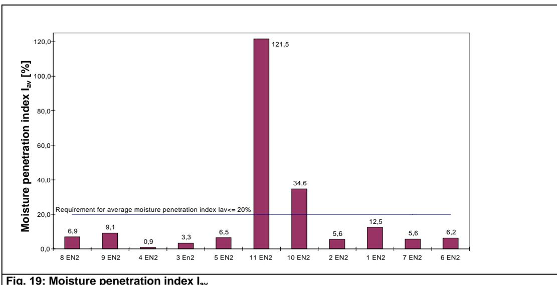
Fig. 19: Moisture penetration index  $I_{av}$
