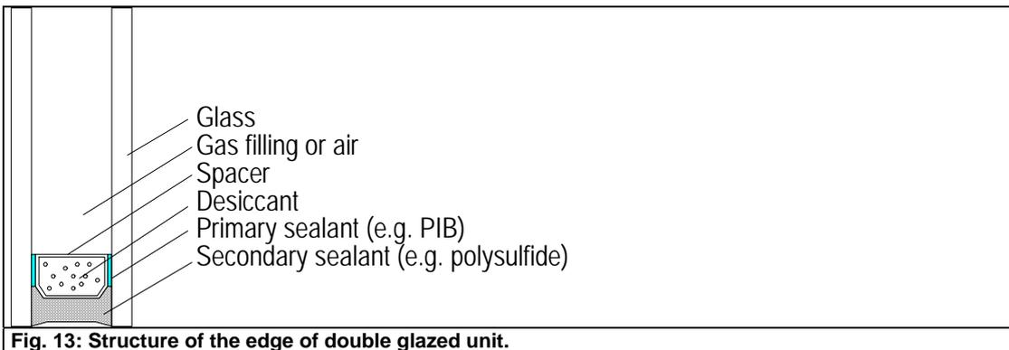
Fig. 13: Structure of the edge of double glazed unit.
