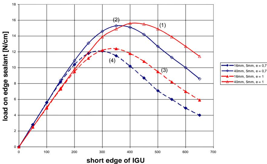
Fig. 31: Load on edge sealant against short edge of IGU for the aspect ratio 0,7 and 1,0 for 5 mm glass panes and interpane separation of 16 mm and 40 mm
