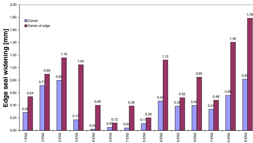
Fig. 22: Widening of the edge sealant after climatic cycles according to DIN EN 1279-2 and -3, measured in the middle of the edge and at the corner of the specimen
