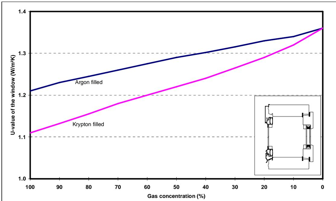
Fig. 17: The effect of the gas concentration in IGU on window U-value. The window size is 1,2 m \* 1,2 m. The low-emissivity coated glass ( $\epsilon=0,04$ ) is used in IGU. The width of the gas gap is 12 mm.
