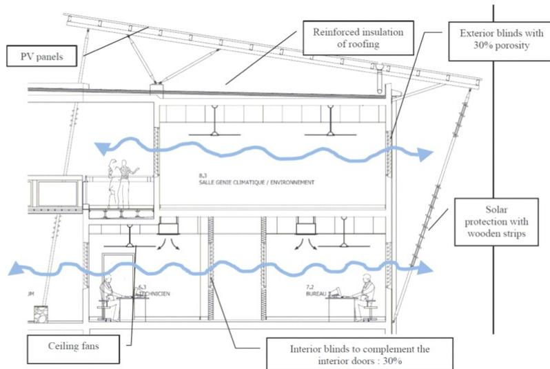
**Figure 3: Passive principle of the ENERPOS building.**
