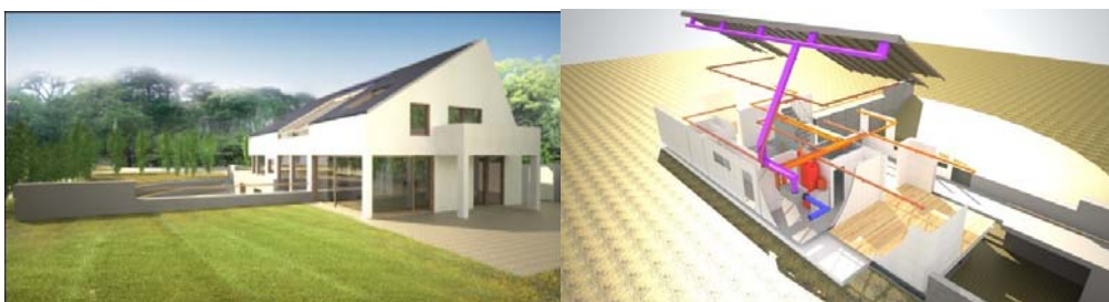
Fig.4 Building Integrated PV Thermal Mechanical Ventilation Heat Recovery System (BIPV/T MVHR) (Source: MEARU Mackintosh School of Architecture).
