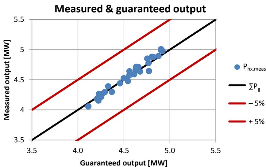
Fig.4. Plot of measured thermal power point against corresponding guaranteed thermal power points. (Source: PlanEnergi)
