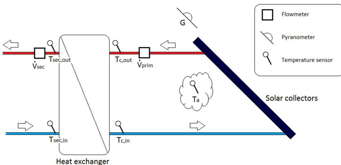
Fig. 2. Schematic drawing showing the measurement points.  $T_{c,out} = T_{prim,in}$  and  $T_{c,in} = T_{prim,out}$ .
