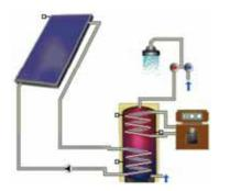
**Figure 44** shows the hydraulic scheme used for the energy calculation for all pumped solar thermal systems and **Figure 45** refers to the thermosiphon systems.
