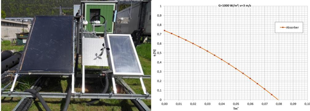
Figure 2: Left - functional model collectors at the outdoor test facility; Right - measured efficiency curve of the large collector.
