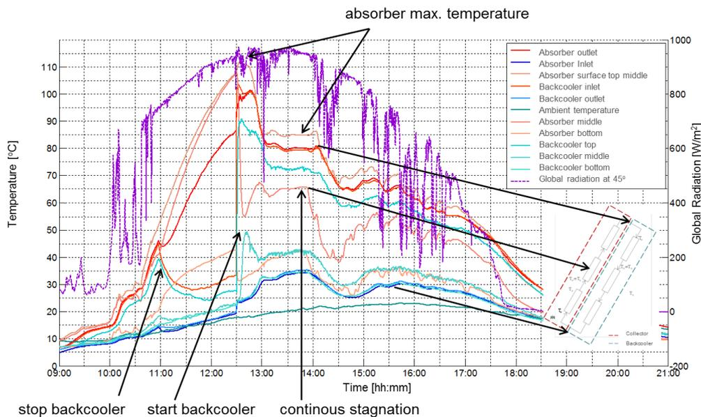
Figure 3: Stagnation test showing the potential of temperature limitation at the absorber.
