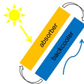
Figure 1: Principle of overheat protection via thermosyphonal backcooling.
