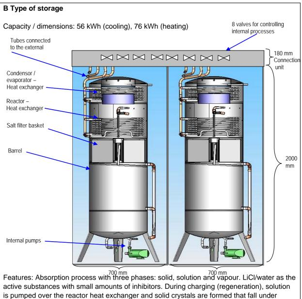
gravity and are collected in a basket. During discharge the solid crystals are dissolved using
