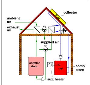
The necessary heat for desorption is delivered by the solar system during summer. Then a conventional solar combisystem is needed just for domestic hot water preparation. With its large collector area (designed for space heating) a conventional solar combisystem has large stagnation time when it can not deliver any solar power. In the described system this time periods are used for the desorption of the adsorption store. This leads to high solar efficency.
