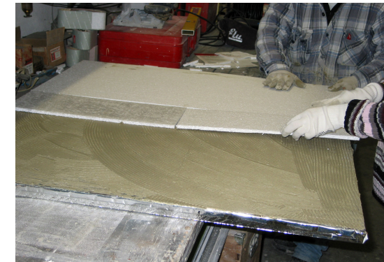
Pre-packing vacuum pack panels in polystyrene
