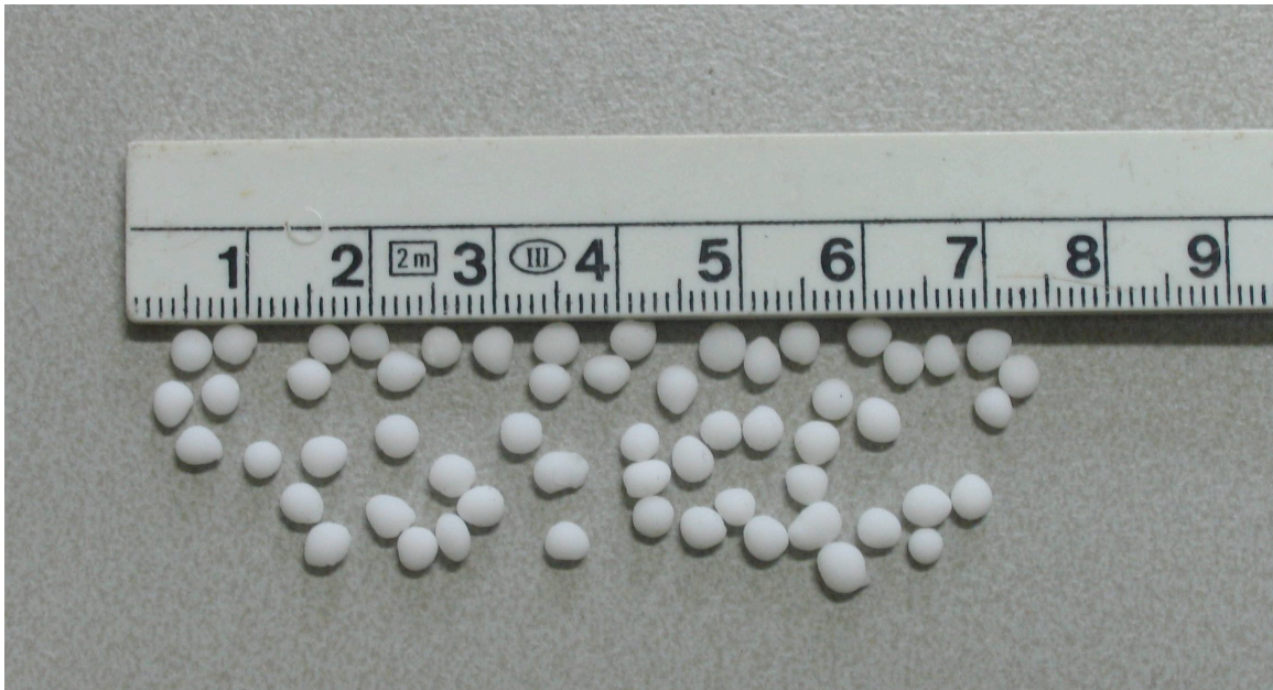
Figure 4: Macro-encapsulated salt hydrate PCM capsules.
