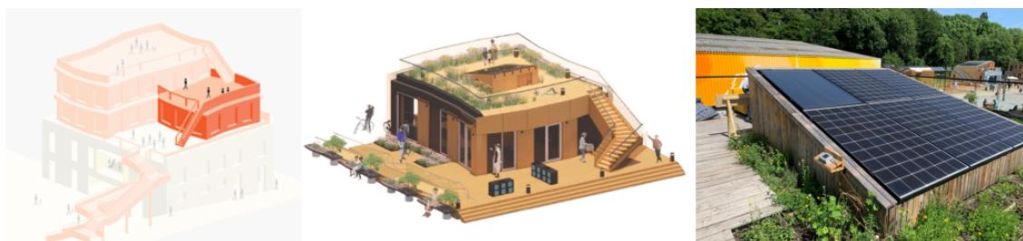
The wood-based building of the VIRTUe team from the Netherlands can be used to add additional floor space to existing buildings. The roof is walkable and includes a PVT field plus a solar collector linked to the house's underfloor heating and cooling system.
