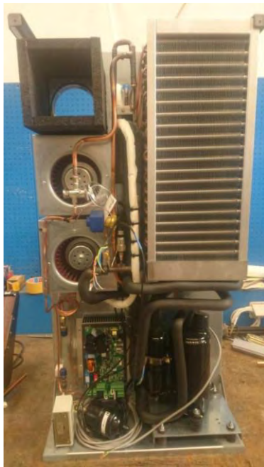
Functional model of outdoor unit with evaporator and CFU simulation
