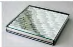
Figure 7: Sample of OKASOLAR 3D in a 3-pane insulating glazing unit, appearance as seen from outside
