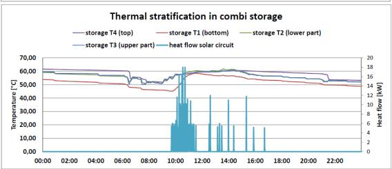
Fig. 10b: Exemplary results for the hybrid heat pump for July 12th, 2011
