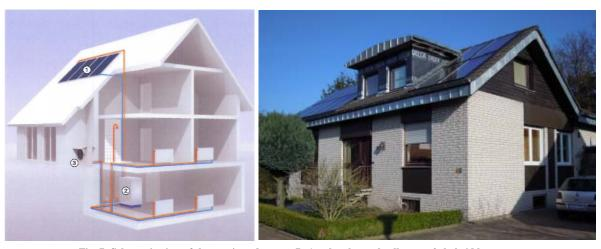
Fig. 7: Schematic view of the monitored system B, 1: solar thermal collectors, 2: hybrid heat pump, 3: external split unit
