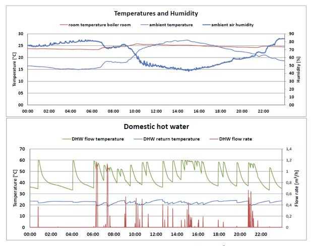
Fig. 10a: Exemplary results for the hybrid heat pump for July  $12^{\text{th}}$ , 2011
