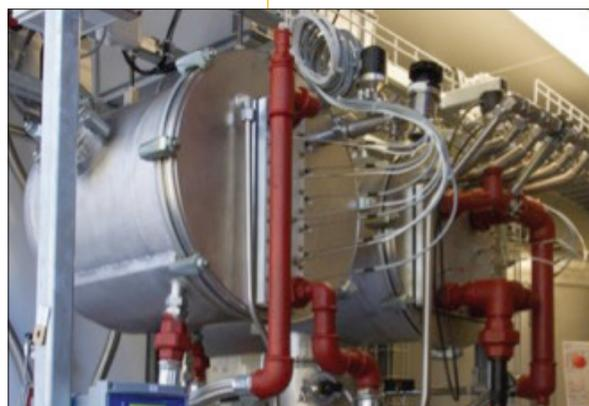
▲ **Figure 1. The COMTES Line B sodium hydroxide heat and mass exchanger installed in the complete demonstration system.**
