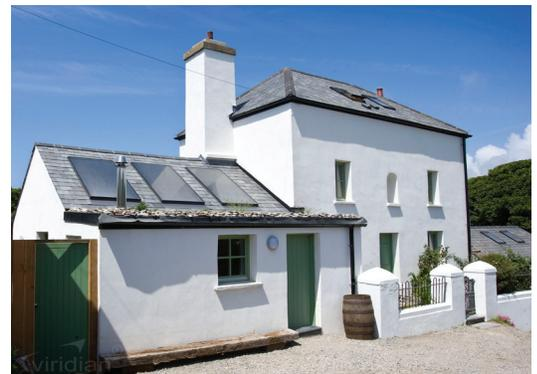
▲ Figure 5. Viridian Solar roof-integrated solar water heating system installed on a Welsh cottage with slate roof.
