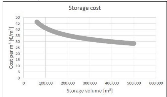
▲ Figure 5. Estimation of the costs for pit heat storage as a function of the size of the storage. (Source: PlanEnergi)
