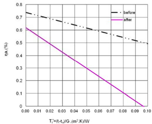
**Fig.6. thermal performance change of UETC**
