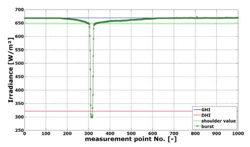
Figure 3-16. Burst (sweep) with sensor signal and the derived GHI, shoulder values, and DHI.
