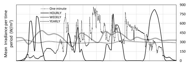
Fig. 2-10. Variability of global irradiance time series at a North American location, as a function of integration time. The figure includes one day of 1-minute data, 4 days of hourly data, 26 weeks of weekly data, and 16 years of yearly integrated data. *Image from Perez et al.* (2016)
