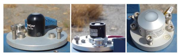
Figure 3-11. Selected photodiode sensors with different diffusor geometries. *Photos from Stefan Wilbert, DLR*
