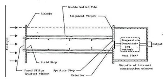
Figure 3-3. Schematic of an Eppley Laboratory, Inc., model normal incidence pyrheliometer (NIP) (Bahm and Nakos 1979). *Image from the former U.S. Energy Research and Development Administration, now DOE*
