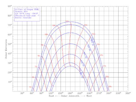
Figure 2-5. Apparent sun path variations during one year in Denver, Colorado. *Image from the University of Oregon Solar Radiation Monitoring Laboratory*(<a href="http://solardata.uoregon.edu/SunChartProgram.php">http://solardata.uoregon.edu/SunChartProgram.php</a>)
