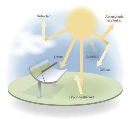
Figure 2-6. Solar radiation components resulting from interactions with the atmosphere. *Image by AI Hicks, NREL*
