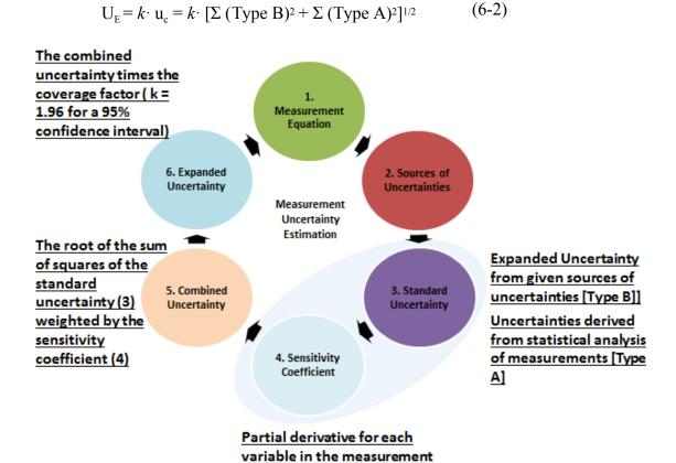
Figure 6-1. Measurement uncertainty estimation flow chart (Habte et al. 2016b)
