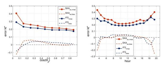
Figure 7-6. Clear-sky forecast error (solid lines for RMSE; dashed lines for mean bias error) as a function of cosine of solar zenith angle (left panel) and hour of the day (right panel) for the forecasts issued by the IFS and SKA NWP models (blue and red lines, respectively). The evaluated period is March 1, 2013–February 28, 2014.
