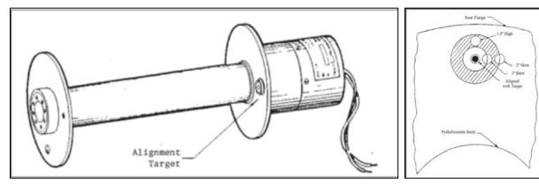
Figure 3-5. Schematics of pyrheliometer alignment diopter configuration including alignment errors for selected positions of the light spot. *Image used with permission from Leonard Micek (Micek 1981)*
