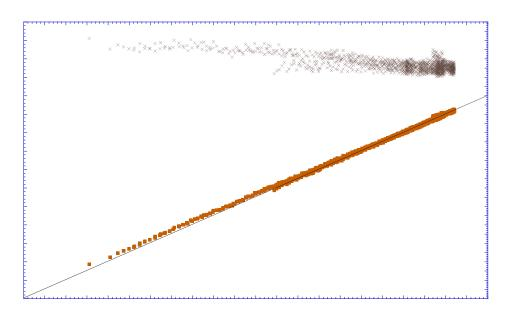
Figure 3-19. Comparison between 1-minute DNI measurements obtained with an EKO MS-05 and an MS-57 reference pyrheliometer at NREL during a 2-day test period
