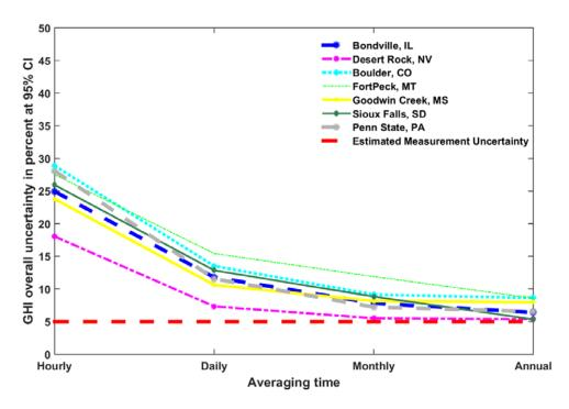
Figure 6-3. Uncertainty estimation of the modeled GHI in the NSRDB (1998–2015) for the 95% confidence interval (CI; *k*≈2) under various time averages at seven National Oceanic and Atmospheric Administration (NOAA)SURFace RADiation (SURFRAD) locations
