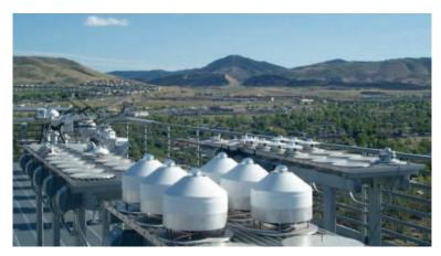
Figure 3-10. Kipp & Zonen model CM22 pyranometers installed in ventilated CV2 enclosures.
