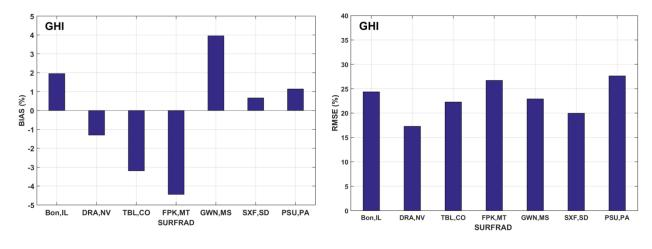
Figure 6-4. Relative bias (left) and RMSE (right); comparison results of modeled data from the NSRDB (1998–2015) relative to irradiance measurements made at seven stations from the NOAA SURFRAD network
