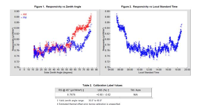
Figure 3-13. Pyrheliometer calibration results summarizing (left) Rs compared to SZA and (right) compared to local standard time. *Image by NREL*
