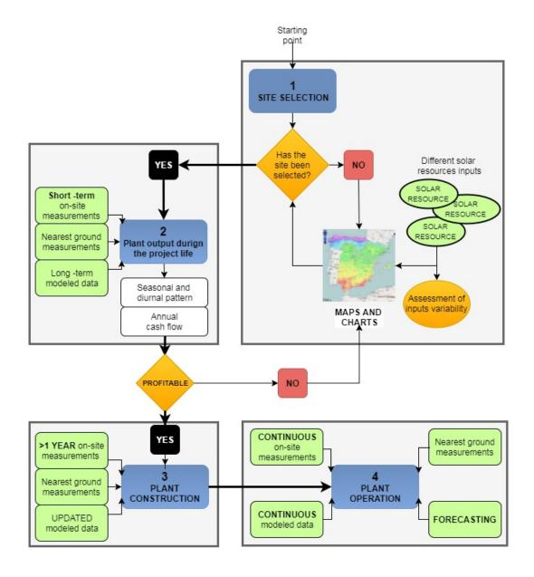
Figure 8-3. Flowchart of the solar radiation data needs (in green) for a solar power project.
