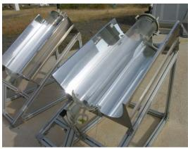
Figure 8-12. CPC photo-reactors installed at PSA for solar water disinfection applications: (left) CPC-SODIS, (right) FITOSOL-2. (Source: PSA, CIEMAT <a href="http://www.psa.es/en/instalaciones/aguas.php">http://www.psa.es/en/instalaciones/aguas.php</a>)
