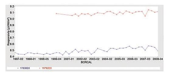
Figure 3-12. Calibration histories for two pyrheliometer control instruments spanning 12 years.
