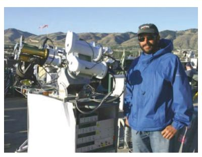
Figure 3-6. Multiple electrically self-calibrating absolute cavity radiometers mounted on solar trackers with control and data acquisition electronics. *Image by NREL*
