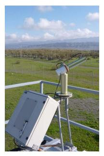
Figure 3-21. AERONET sun photometric station at the Plataforma Solar de Almería. *Photo from DLR*
