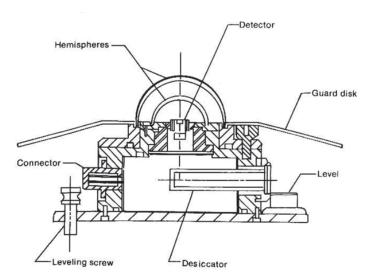
Figure 3-9. Schematic of the Eppley Laboratory, Inc., Precision Spectral Pyranometer (PSP) model.
