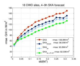
Figure 7-7. RMSE of various versions of the SKA forecasts as a function of the standard deviation of kt\*meas([red] SKA: nearest grid point, [dark blue] SKA20x20 averaged throughout 20-by-20 grid points, [light blue] SKAav 5 h sliding mean of clear-sky index of the average throughout 20-by-20 grid points, and [green] SKAav, LR.kt\*: linear regression of kt\* applied to SKAAV). The evaluated period is April 3, 2013–February 28, 2014; training set: last 30 days, all sites.
