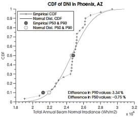
Figure 8-9. (Left) Annual GHI data fitted to a normal distribution (solid line) for Phoenix, Arizona. (Right) Same as left plot but for DNI. Note that each gray circle covers a marker (+).
