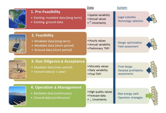
Figure 8-2. Solar radiation needs at four stages of a solar power project. Pictures from www:
