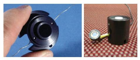
Figure 3-1. (Left) Thermopile assembly used in an Eppley Laboratory, Inc., model precision spectral pyranometer (PSP); (right) typical photodiode detector. *Photograph used with permission from LI-COR*, *Inc.*
