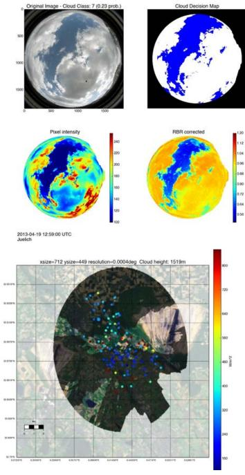
Figure 7-2. Cloud information from sky imagers: upper left, original images; upper right, cloud decision map; middle left, pixel intensity; middle right, red-blue ratio, corrected with a clear-sky library; bottom, shadow map with irradiance measurements. Sky image and irradiance measurements were taken in Jülich, Germany, on April 9, 2013, at 12:59 UTC in the framework of the HOPE campaign (Macke and HOPE-Team 2014). Images from the University of Oldenburg
