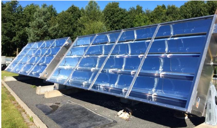
Fig. 8 Photo of the new CPC solar collectors and the test rig.
