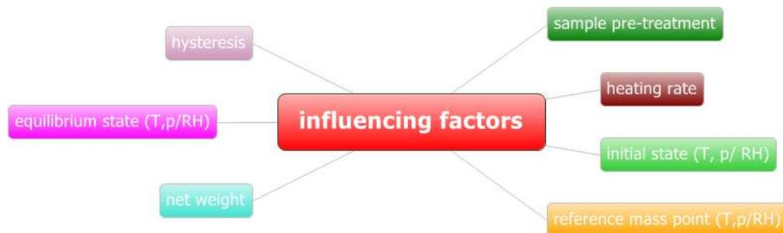
Figure1: Influencing factors for water adsorption measurements [1].
