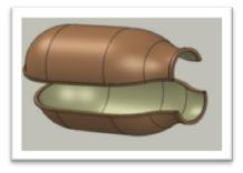
No internal lining will be necessary. The shells can be welded by means of hot-plate, vibration welding or infrared radiation. Welding coefficients are quite strong. This will enable to make a lightweight but pressure resistant tank. The water temperatures are moderate and do not negatively impact the pressure resistance of these engineering materials. The materials used have to be certified according to NSF 61.
