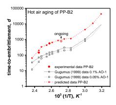
morphology adding a ß-nucleating agent. For the novel PP grades a PE80 classification was achieved providing a long-term strength of components for pressure applications. Using a unique aging characterization approach based on micro-sized specimen, a comprehensive set of aging data was established. For the extrapolation of time-to-embrittlement data at enhanced temperatures (115 and 135°C) to service relevant temperatures (< 100°C) theoretical and empirical models were used.
