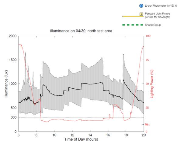
Figure 3. Top: Floor plan layout of furniture, work plane sensors, shades, and light fixtures in the north zone. Bottom: Minimum, average, and maximum work plane illuminance (lx) and average dimming level (%) in the north zone of the new building on a sunny day.
