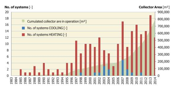
**Figure 40:** Solar district heating and cooling in Europe – annual achievements and cumulated area in operation by end of 2014 (*Data source: Jan-Olof Dalenbäck - Chalmers University of Technology, SE*)
