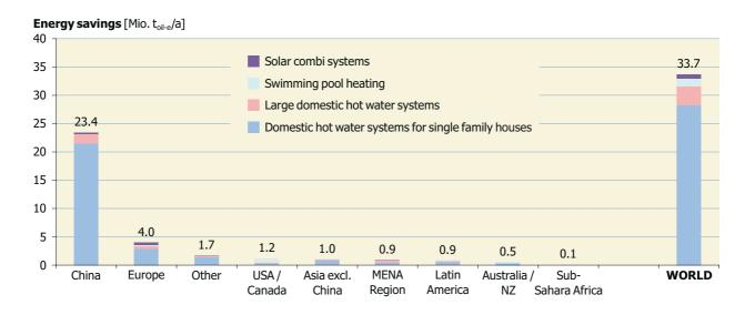
Figure 32: Annual energy savings in oil equivalent by unglazed and glazed water collectors in operation by end of 2013
