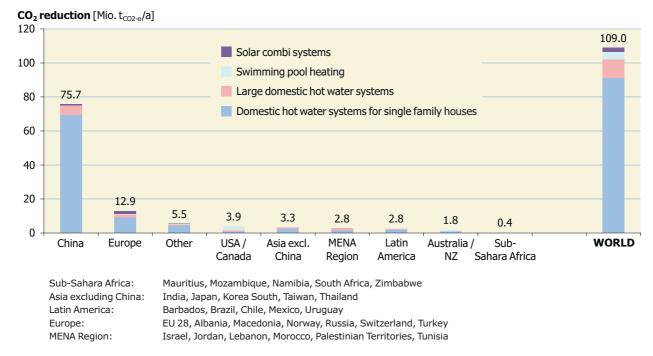
Figure 33: Contribution to CO<sub>2</sub> reduction by unglazed and glazed water collectors in operation by end of 2013
