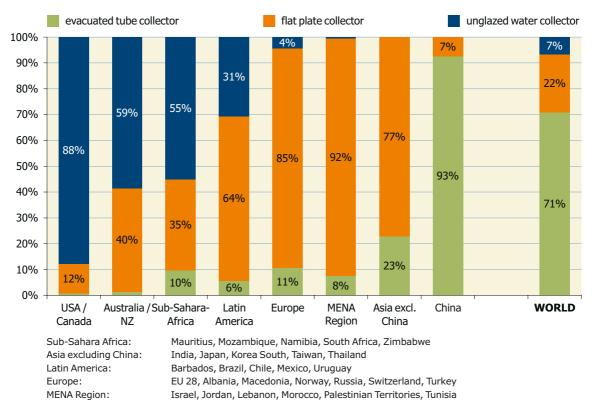
**Figure 34:** Distribution by type of solar thermal collector for the total installed water collector capacity in operation by the end of 2013
