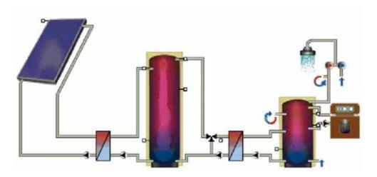
Figure 47: Hydraulic scheme of the domestic hot water pumped reference system for multifamily houses
