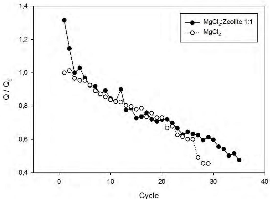
Figure 7: Decrease in reactivity of  $\text{MgCl}_2 \cdot 6 \text{ H}_2\text{O}$  and a zeolite composite, respectively, during subsequent hydration/dehydration cycles. The amount of heat released during hydration of the sample was measured.
