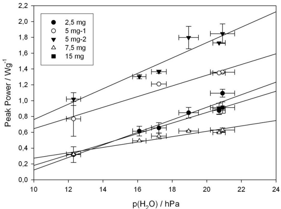
Figure 3: Dependency of the peak heat flux observed during hydration of  $\text{MgCl}_2 \cdot 2 \text{ H}_2\text{O}$  on water vapour partial pressure and sample size.
