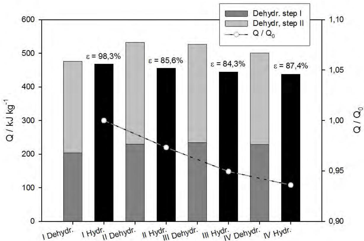
Figure 8: Heat quantities during dehydration and hydration, cycle efficiency and cycling stability using the transition of MgCl<sub>2</sub> \* 6 H<sub>2</sub>O  $\rightarrow$  MgCl<sub>2</sub> \* 2 H<sub>2</sub>O + 4 H<sub>2</sub>O of a MgCl<sub>2</sub> \* 6 H<sub>2</sub>O : Graphite (1:1) composite.
