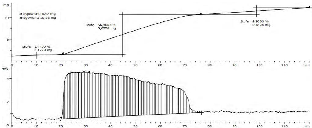
Figure 2: Hydration TGA/DSC plot of  $\text{MgCl}_2 \cdot 2 \text{H}_2\text{O}$  to  $\text{MgCl}_2 \cdot 6 \text{H}_2\text{O}$  (35°C,  $p(\text{H}_2\text{O}) \sim 2 \text{kPa}$ )
