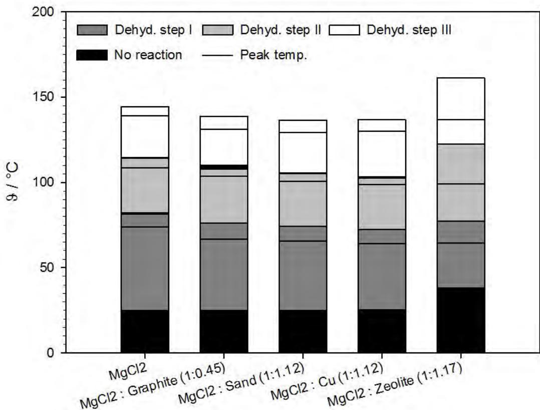
Figure 5: Influence on observed reaction temperatures of different additives.
