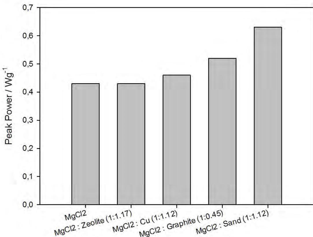
Figure 6: Peak heat fluxes observed during dehydration (step II) of the different composites, normalized to  $\text{MgCl}_2 \cdot 6 \text{ H}_2\text{O}$  content.
