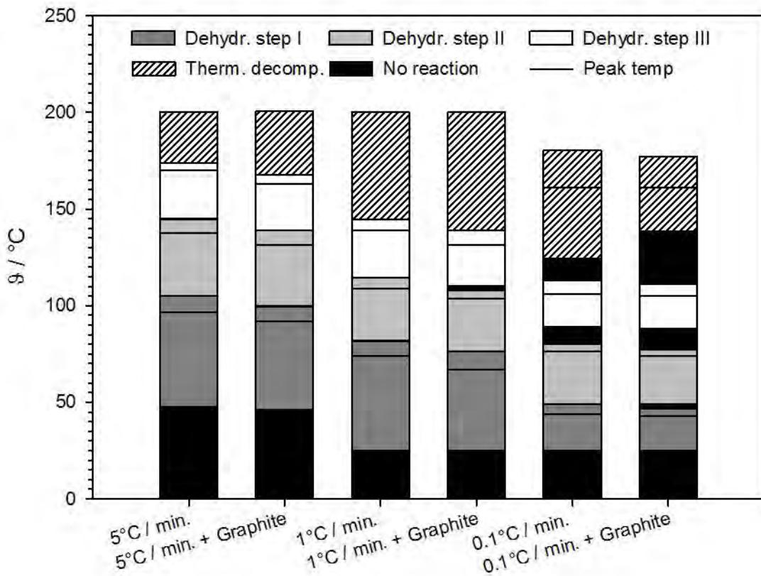
Figure 4: Reaction temperatures observed during dehydration of  $\text{MgCl}_2 \cdot 6 \text{ H}_2\text{O}$  and a  $\text{MgCl}_2 \cdot 6 \text{ H}_2\text{O} : \text{graphite}$  composite (1 : 0.45) at different heating rates, 25 – 200°C.
