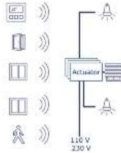
Figure 9. Centralized Control System (Source:EnOcean Alliance).
